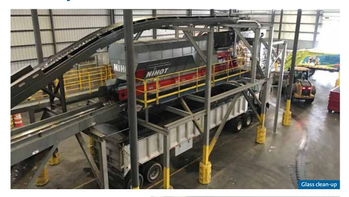
The SDi is a flexible semi-mobile windshifter, aimed at operators who require a high-performing, versatile machine that remains easy to transport. This is of high value due to following characteristics:
