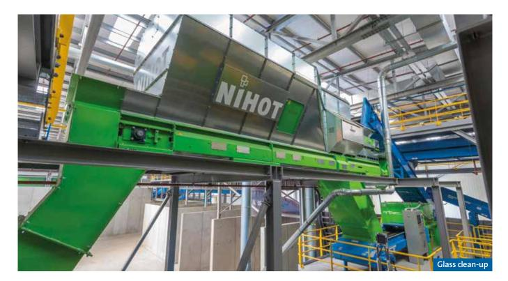
The Nihot SDi is able to generate a precise heavy / light separation for a wide range of input materials, including removing contaminants from high-value commodities in an MSW stream. Whether you're removing inerts from biomass or compost, or processing glass, incinerator ash or Automotive Shredder Residue (ASR), the SDi will be of great value.
