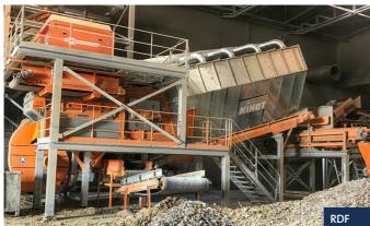
The SDX is a windshifter dedicated for RDF/SRF production plants, using industry-leading negative pressure technology to remove inert from the waste stream for the protection of secondary shredders.
