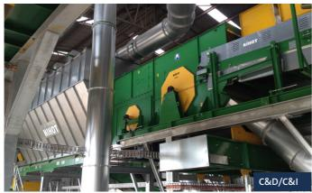
The DDS is the ideal solution for a three-way separation. Input material is separated into a heavy, mid-heavy and light fraction. The three-way fraction is created by primary and secondary fans in combination with two drums.
