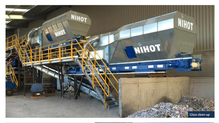
The SDi windshifter is able to generate a precise heavy / light separation for a wide range of input materials. Whether you are removing inerts from biomass or compost, or processing glass, incinerator ash or Automotive Shredder Residue (ASR), the SDi will be of great value.
