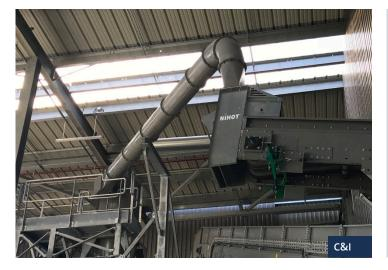
The WSS windshifter is the ideal solution for any operation, but especially in removing plastic film from MSW, packaging waste and PET.
