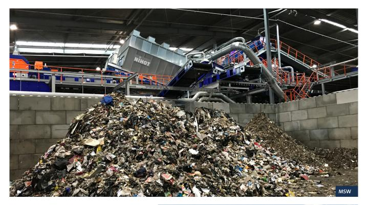
The SDS windshifter separates all kind of waste types into two fractions, heavy and light. The robust construction and fool proof functionality guarantee a long lasting and trouble-free operation.
