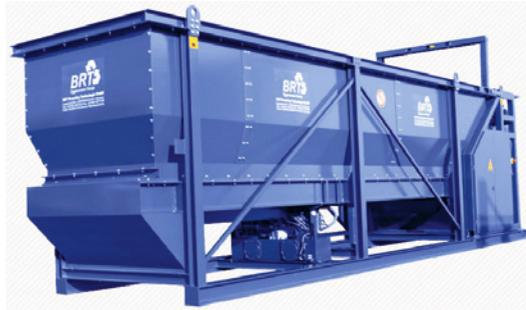
Sliders open bags of waste automatically, eliminating the need for human contact with potentially hazardous materials
