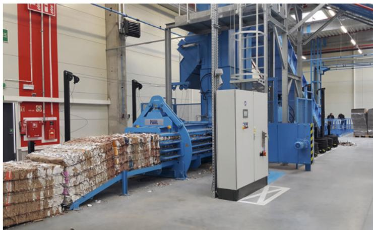
Large presses compress and bale materials as part of the recycling process
